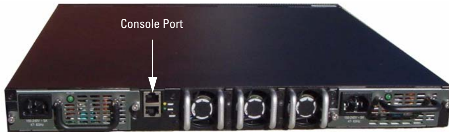
Figure 3. Connecting to the Console Port
